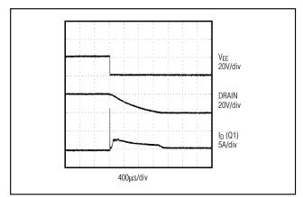
Figure 8. Voltage Step-On Input Supply
