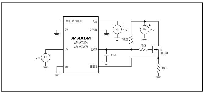
Figure 1b. Test Circuit 2
