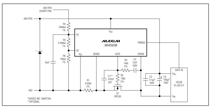
Figure 6a. Inrush Control Circuitry
