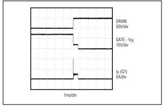
Figure 7b. Short-Circuit Protection Waveform
