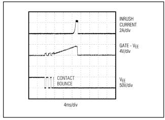
Figure 7a. Startup Into a Short Circuit
