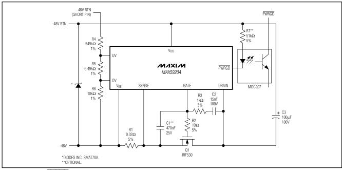
Figure 14. Using PWRGD to Drive an Optoisolator
