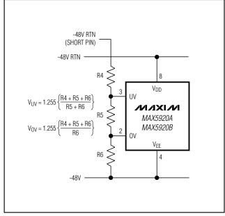
Figure 11. Undervoltage and Overvoltage Sensing
