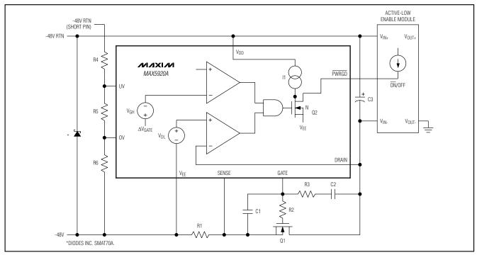
Figure 13. Active-Low Enable Module
