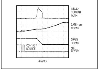
Figure 6b. Input Inrush Current
