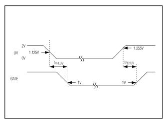
Figure 3. UV to GATE Timing
