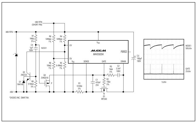
Figure 10. Automatic Restart After Current Fault
