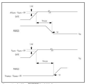
Figure 5b. GATE to PWRGD/PWRGD Timing
