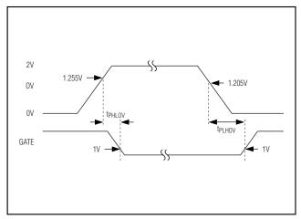
Figure 2. OV to GATE Timing
