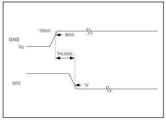
Figure 4a. SENSE to GATE Timing
