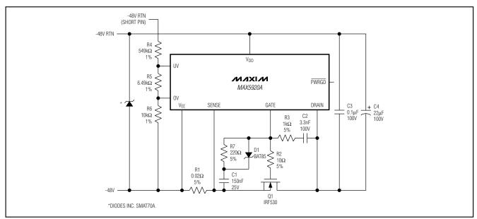
Figure 9. Circuit for Input Steps with Small C1
