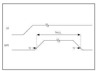
Figure 4b. Active Current-Limit Threshold
