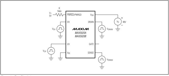
Figure 1a. Test Circuit 1
