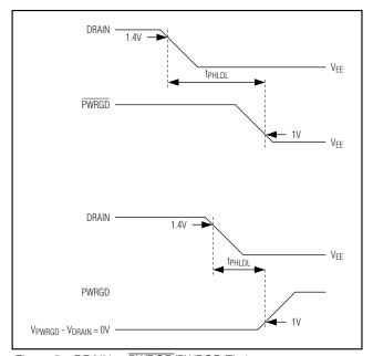
Figure 5a. DRAIN to PWRGD/PWRGD Timing
