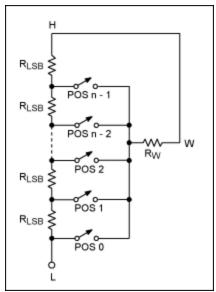
Figure 2. Digital potentiometer resistor model.
