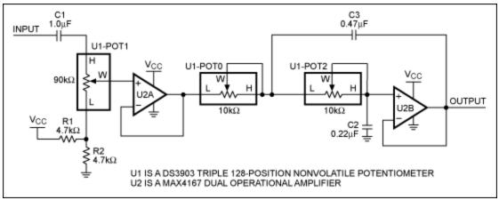
Figure 1. Audio range lowpass filter using a DS3903.
