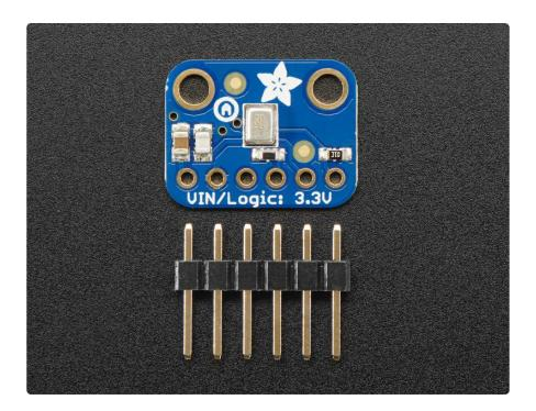
The microphone is a single mono element. You can select whether you want it to be on the Left or Right channel by connecting the Select pin to power or ground. If you have two microphones, you can set them up to be stereo by sharing the Clock, WS and Data lines but having one with Select to ground, and one with Select to high voltage.
