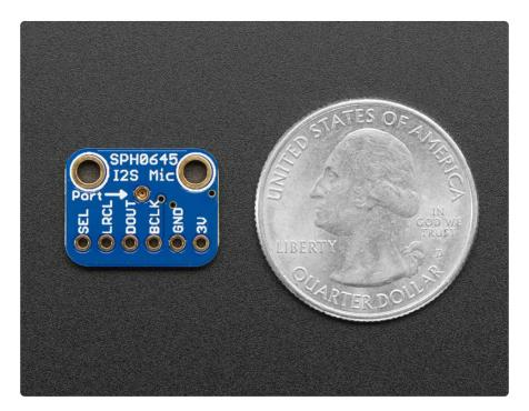
This I2S MEMS microphone is bottom ported, so make sure you have the hole in the bottom facing out towards the sounds you want to read. It's a 1.6-3.3V device only, so not for use with 5V logic (its really unlikely you'd have a 5V-logic device with I2S
