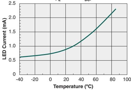
**Typical  $I_F$  for Switch Dropout vs. Temperature**
