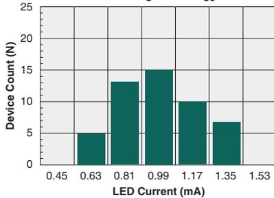
**Typical  $I_F$  for Switch Dropout**
