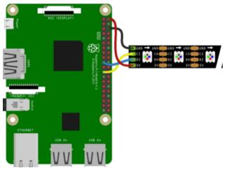
Pi 5V to LED 5V Pi GND to LED GND Pi MOSI to LED DI Pi SCLK to LED CI
