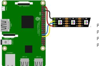
Pi 5V to LED 5V Pi GND to LED GND Pi GPIO5 to LED DI Pi GPIO6 to LED CI
