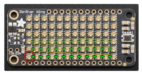
We refer to this layout as row major and progressive. Row major means the pixels are arranged in horizontal lines (the opposite, in vertical lines, is column major). Progressi ve means each row proceeds in the same direction. Some matrices will reverse direction on each row, as it can be easier to wire that way. We call that a zigzag layout.
