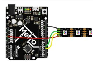
If using a one-meter strip or less, it's usually OK to power off the microcontroller's 5V pin. Here's how it might look on an Arduino Uno or Adafruit Metro board:
