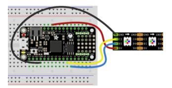
Board USB to LED 5V Board GND to LED GND Board MO to LED DI Board SCK to LED CI
