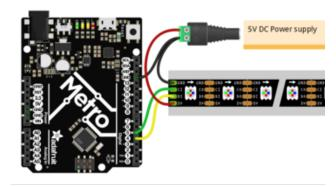
The simplest wiring is if you can power the strip off of the microcontroller board itself. This is fine for small projects (one or two dozen DotStars max) because we don't light up a lot of LEDs at once.
