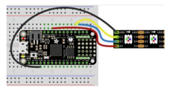
Board USB to LED 5V Board GND to LED GND Board D5 to LED DI Board D6 to LED CI
