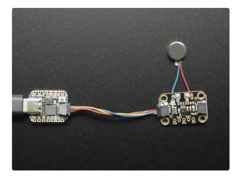
The DRV2605 from TI is a fancy little motor driver. Rather than controlling a stepper motor or DC motor, it's designed specifically for controlling haptic motors - buzzers and vibration motors. Normally one would just turn those kinds of motors on and off, but this driver has the ability to have various effects when driving a vibe motor. For example, ramping the vibration level up and down, 'click' effects, different buzzer levels, or even having the vibration follow a musical/audio input.
