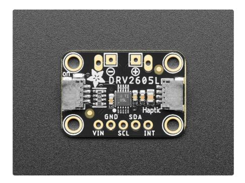
According to the product page, it can be used with both LRA (Linear Resonance Actuator) and ERM (Eccentric Rotating Mass) type motors <u>but we have only used it</u> with our little vibration pancake ERM. ()
