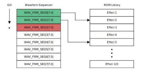
You access the Waveform Sequencer by using the sequence property and providing an index for the slot location. To specify the effect, use the special Effect class provided in the library, giving it the effect number.
