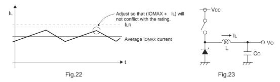
Adjust so that (IOMAX + DIL) will not conflict with the rating. At this time, DIL can be obtained according to the formula shown below.
