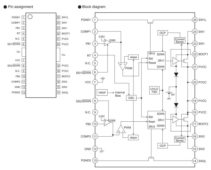
Fig.18 Pin assignment / Block diagram
