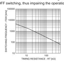
Fig.25 RT vs. Switching frequency
