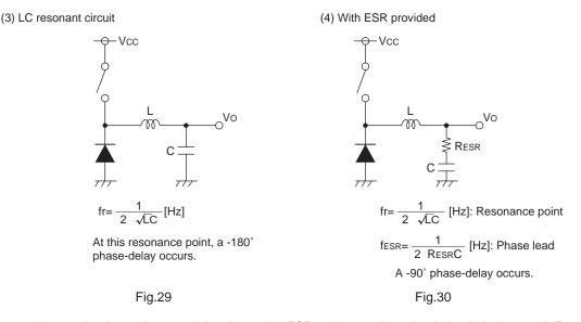
According to changes in phase characteristics due to the ESR, only one phase lead should be inserted. For this phase lead, select either of the methods shows below.
