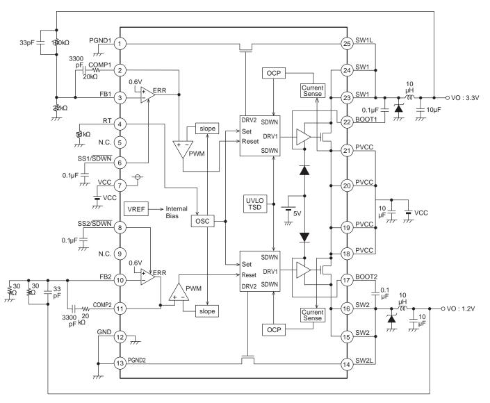
Fig.19 Typical application circuit
