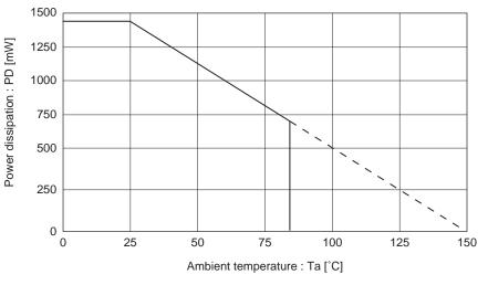
Fig.37 Thermal derating characteristics
