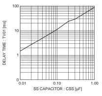
Fig.26 SS capacitance vs. Delay time
