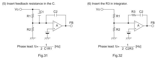
For the purpose of canceling the LC resonance, the frequency to insert the phase lead should be set close to the LC resonant frequency.
