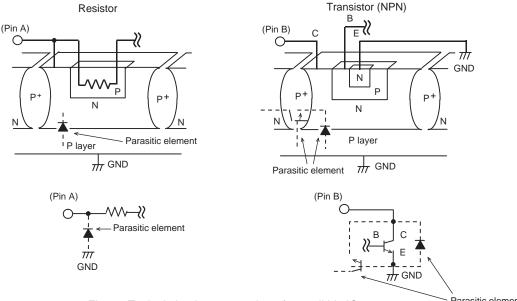
Fig.35 Typical simple construction of monolithic IC
