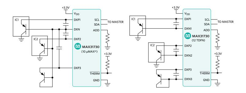
Figure 10. Remote Temperature Sensor Monitoring the Temperature of a Sensing Transistor (or Thermal Diode) on the Die of an External IC
