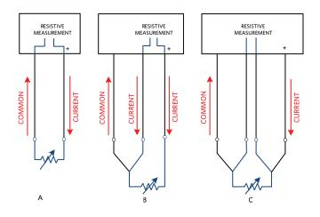
Figure 4. Two-Wire, Three-Wire, and Four-Wire RTD
