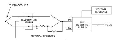
Figure 2. Thermocouple-to-Digital Compensation Circuit
