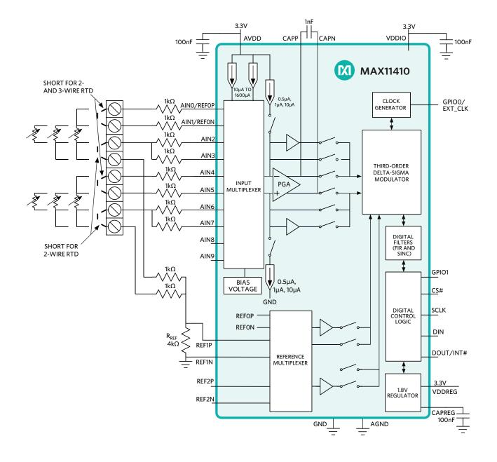
Figure 5. Dual RTD Measurement Circuit
