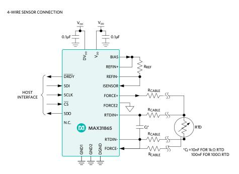
Figure 6. MAX31865 in Two-/Three-/Four-Wire Configurations
