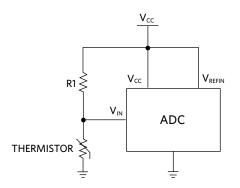
Figure 7. Thermistor-to-ADC Interface
