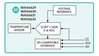
Figure 9. Local Temperature Sensor with an Internal ADC
