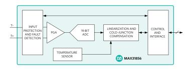
Figure 3. MAX31856 Simple Block Diagram
