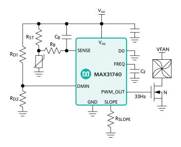
Figure 8. Two-Wire Fan-Speed Controller
