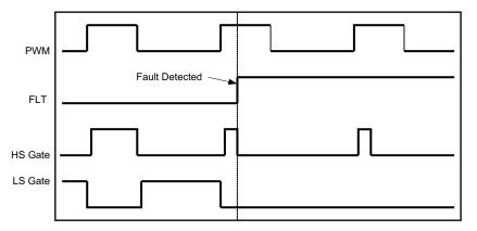
Figure 3. High-side Overcurrent Fault Response
