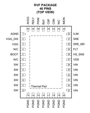
The thermal pad is also an electrical ground connection.
