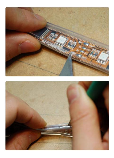
Pull off the thin rubber piece between the cuts:
