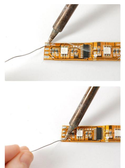
Start by soldering a red wire to the +5V power line:
