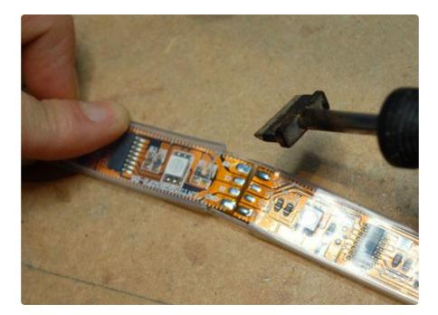
Cut the remaining rubber underneath with scissors:
