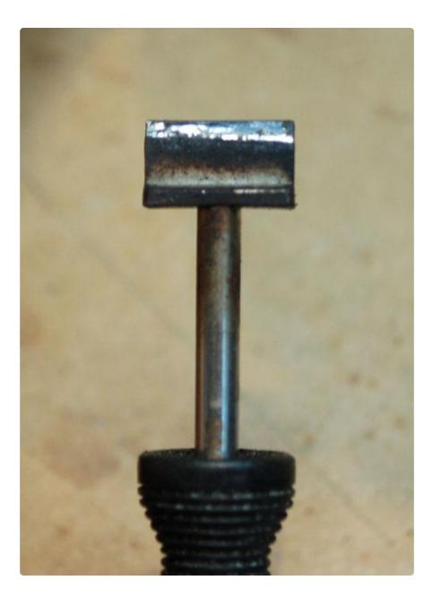
Using an X-acto knife, cut two slices from the top on either side of the solder connection:
