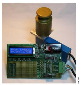
Figure 2. Weigh Scale System Using the AD7191
