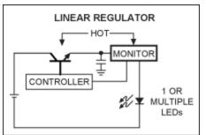
Figure 1a. A simple linear regulation scheme experiences power losses due to both the regulator and the current-setting resistor. The advantages of this circuit are its simplicity and the fact that it generates no EMI. The circuit can, however, only lower voltage and it does generate some heat.
