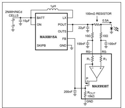
Figure 2. Working from Figure 1b, a current-sense amplifier such as the MAX9938T reduces the power losses in the current-sensing resistor to just a few tens of milliwatts vs. hundreds of milliwatts, or more, for the previous schemes in Figure 1.
