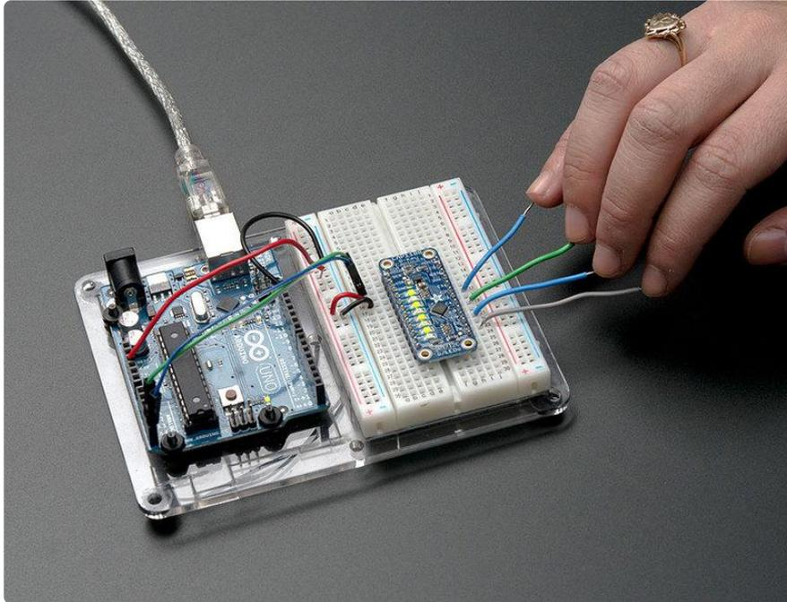
Add lots of touch sensors to your next microcontroller project with this easy-to-use 8-channel capacitive touch sensor breakout board, starring the CAP1188. This chip can handle up to 8 individual touch pads, and has a very nice feature that makes it stand out for us: it will light up the 8 onboard LEDs when the matching touch sensor fires to help you debug your sensor setup.
