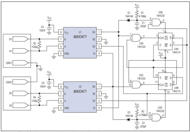
Figure 1. This RS-422 repeater draws only 3µA of standby current.
