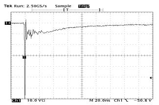
Figure 1. IEC61000-4-2 +8 KV Contact ESD **Clamping Voltage**
