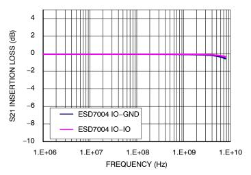
Figure 15. ESD7004 Insertion Loss
