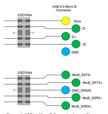
Figure 17. USB3.0 Micro B Connector Layout Diagram
