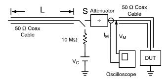
Figure 8. Simplified Schematic of a Typical TLP System
