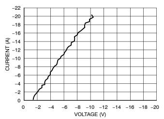
Figure 7. Negative TLP I-V Curve
