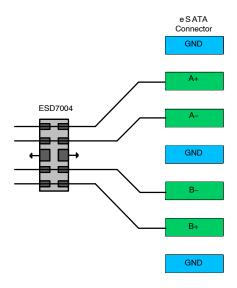
Figure 19. eSATA Layout Diagram
