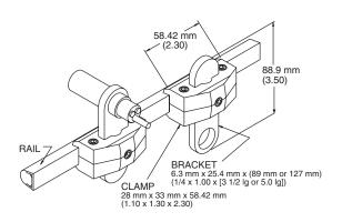
AC227 Large, right-angle, stainless, mounting bracket (for 18 mm barrel sensors)
