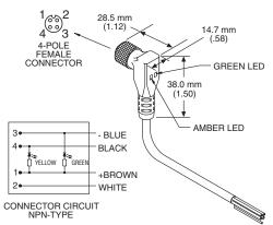
AC127 Straight, M12 micro, 4-conductor, connector/cable assembly, 5 m (16'), with built-in LEDs (for barrel connector-style sensors)
