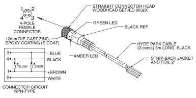
AC130 Straight, M12 micro, 4-conductor, connector/cable assembly, 5 m (16') (for flat-profile connector-style sensors)
