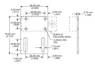
Small, right-angle, stainless, mounting bracket (for 18 mm barrel sensors)
