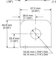
AC228 Small, right-angle, stainless, mounting bracket (for 18 mm barrel sensors)
