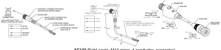
**AC132** Right-angle, M12 micro, 4-conductor, connector/ cable assembly, 5 m (16') (for flat-profile connector-style sensors)
