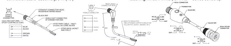
**AC132** Right-angle, M12 micro, 4-conductor, connector/cable assembly, 5 m (16') (for flat-profile connector-style sensors)
