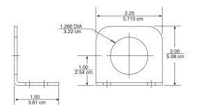
**Model AC213,** Stainless and Teflon, remote sensing probe mounting bracket
