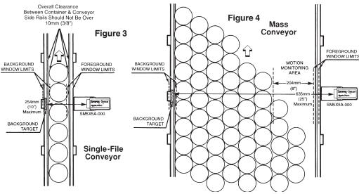
place a container on the conveyor against the rail nearest to the sensor with the main body area directly in front of the sensor and press the LIMITS push-button once. Again, while the push-button is depressed, the LED is amber. Upon release of the push-button, the LED turns green indicating the background and foreground window limits have been successfully set. If 30 seconds elapse before the foreground window limits are set, the limits revert back to the previous settings.
