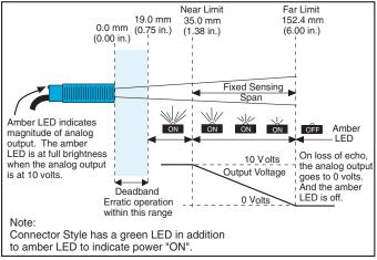
Note: The Cable style sensors have an amber signal LED only; no green LED.
