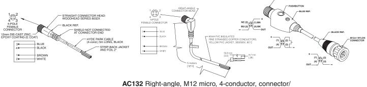
AC132 Right-angle, M12 micro, 4-conductor, connector/ cable assembly, 5 m (16') (for flat-profile connector-style sensors)
