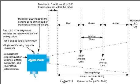
analog signal will go to the minimum or maximum value depending on the position of configuration Switch 2. When the sensor again receives echos from within its sensing range, the analog signal is updated to a value indicating the object's present position relative to the span limits.
