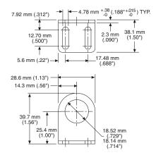
AC231 Straight, stainless mounting bracket (for flat-profile sensors)
