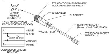
AC130 Straight, M12 micro, 4-conductor, connector/cable assembly, 5 m (16') (for flat-profile connector-style sensors)
