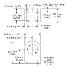
**AC231** Straight, stainless mounting bracket (for flat-profile sensors)
