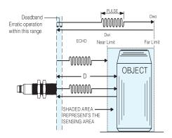
During operation, the calculated distance (D) between the sensor and the object is compared to the distances between the sensor and the fixed window limits. These limits are shown in the illustration as Dwi and Dwo. If D is at or within the limits, an output change takes place and remains unchanged until the echo either does not return or it returns from outside the fixed limits.
