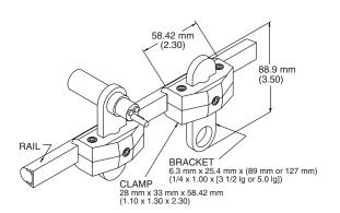
AC227 Large, right-angle, stainless, mounting bracket (for 18 mm barrel
