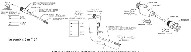
AC132 Right-angle, M12 micro, 4-conductor, connector/cable assembly, 5 m (16') (for flat-profile connector-style sensors)
