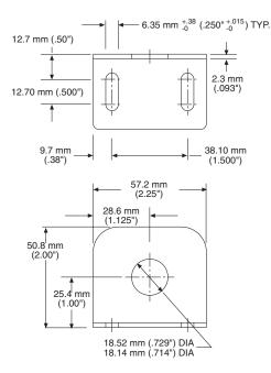
AC228 Small, right-angle, stainless, mounting bracket (for 18 mm barrel sensors)
