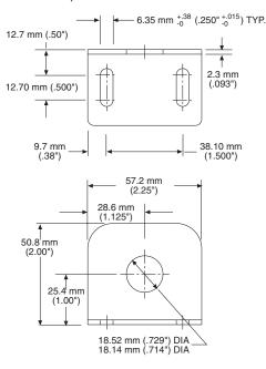
AC228 Small, right-angle, stainless, mounting bracket (for 18 mm barrel sensors)
