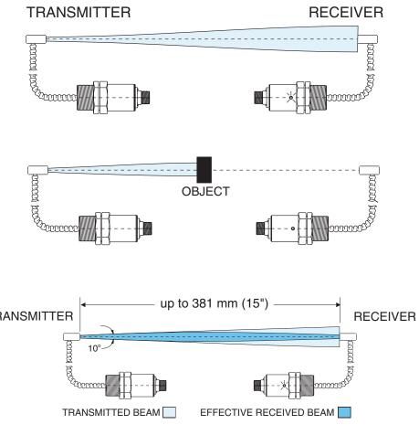
Figure 1, Thru-beam Pattern and Range
