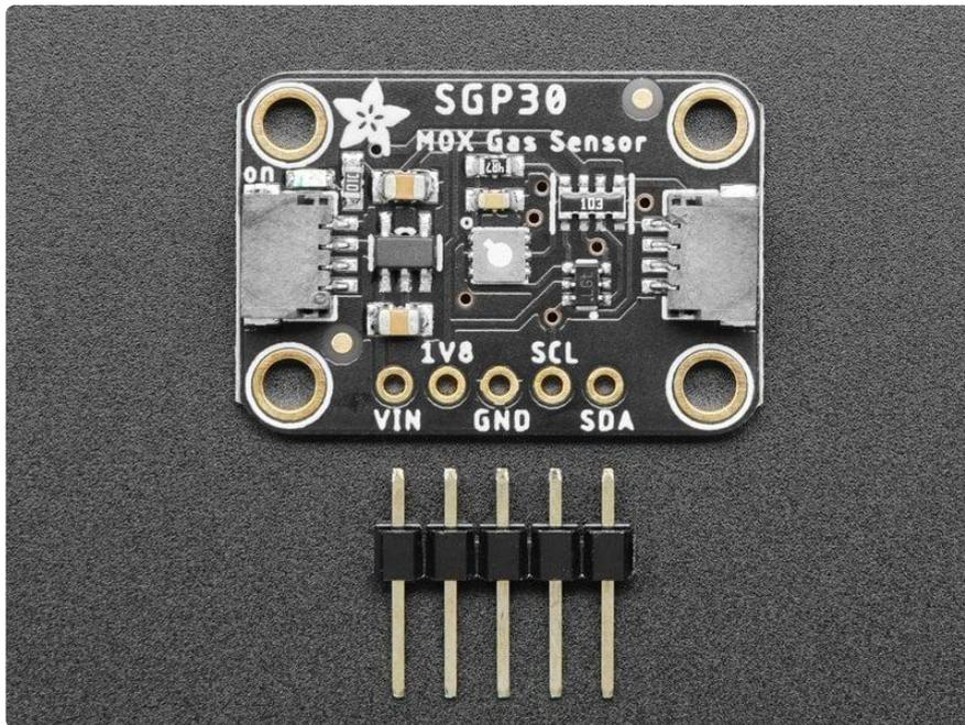
The SGP30 has a 'standard' hot-plate MOX sensor, as well as a small microcontroller that controls power to the plate, reads the analog voltage, tracks the baseline calibration, calculates TVOC and eCO<sub>2</sub> values, and provides an I<sup>2</sup>C interface to read from. Unlike the CCS811, this sensor does not require I<sup>2</sup>C clock stretching.
