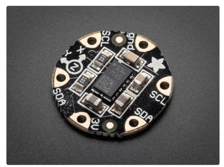
First let's get things moving. The <u>FLORA LSM303</u> () contains an accelerometer, which is great for detecting your dance moves, footsteps, or roller coaster rides. We've used it in the hem of the <u>Sparkle Skirt</u> () and on <u>3D printed wristband</u> () to flash some neopixels when you walk or shimmy.
