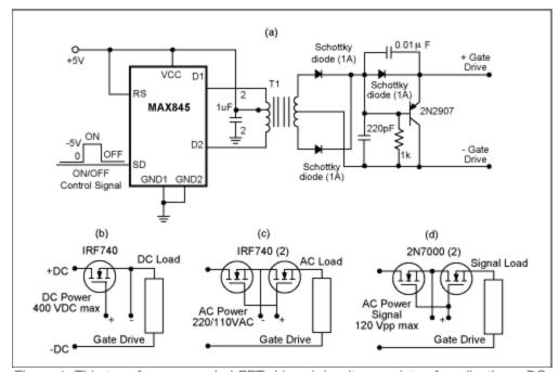
Figure 1. This transformer-coupled FET driver (a) suits a variety of applications: DC power and load (b);
