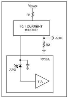
Figure 1. Schematic for a typical APD current monitor.
