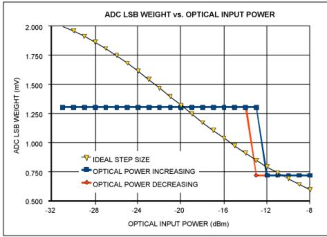
Figure 3. A typical APD monitor's the ideal ADC LSB weight and actual calibrated weights.
