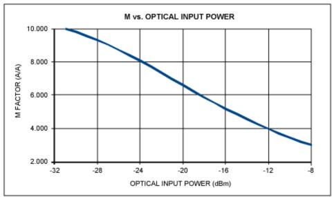
$V_{ADV} = I_{APD} \times (1/10) \times R2 = P_{RX} \times M \times \eta \times (1/10) \times R2$
