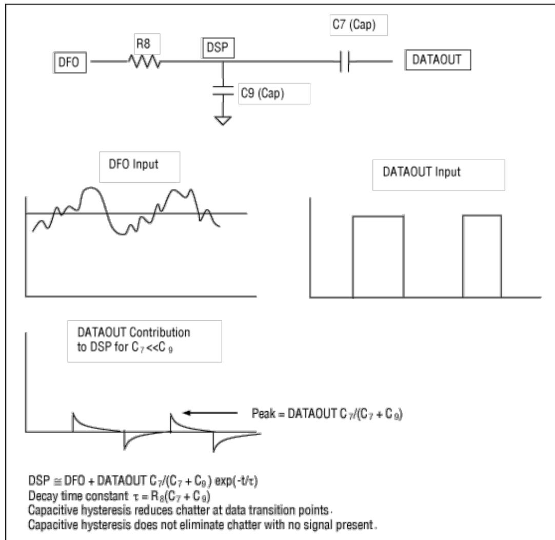
Figure 11. Capacitive hysteresis circuit and waveforms.
