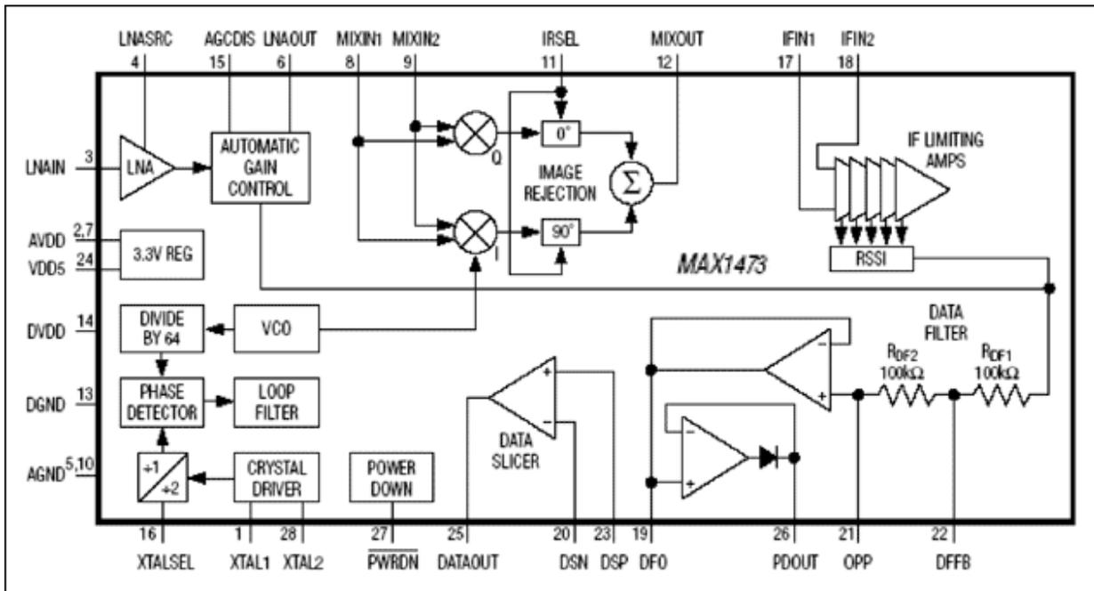
Figure 2. Block diagram of the MAX1473 ASK receiver.
