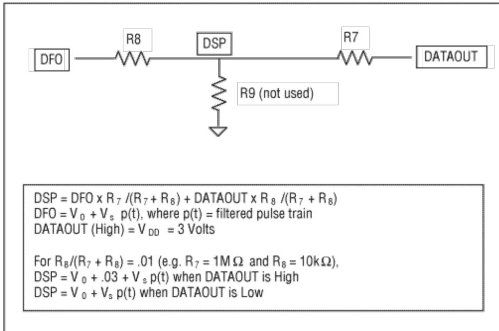
Figure 10. Resistive hysteresis circuit for squelch function.
