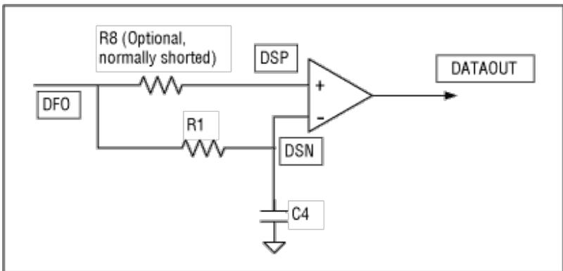
Figure 4. Fundamental data-slicing circuit.
