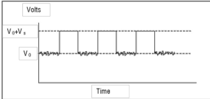
Figure 1. ASK demodulator output.
