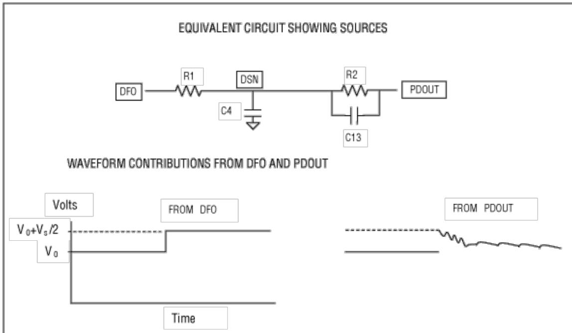
Figure 6. Circuit and waveforms for rapid threshold formation.
