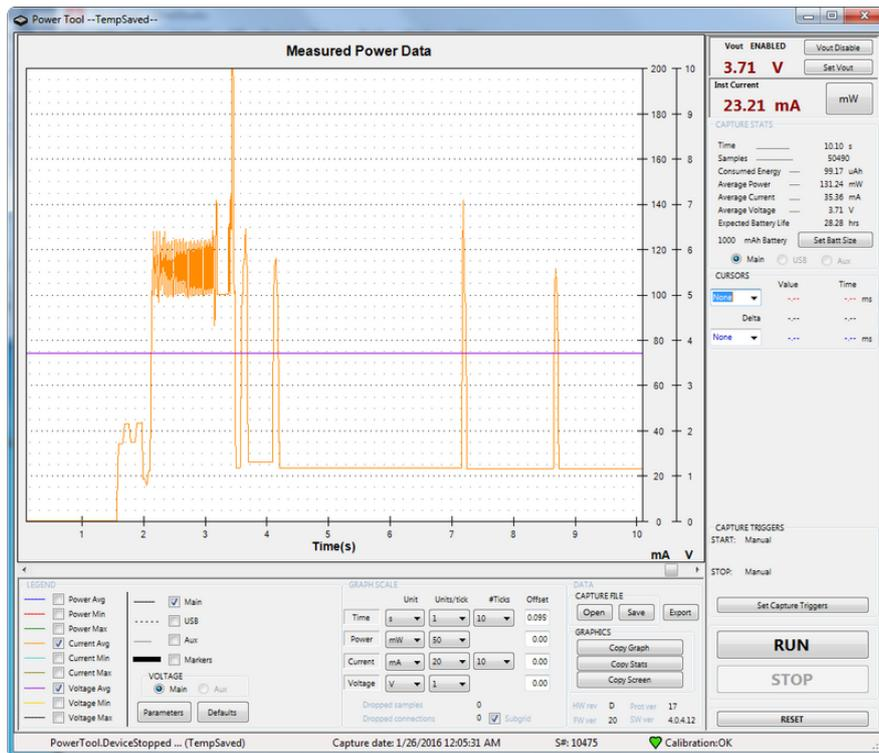
Note that 10mA or so is for the ATSAM chip, so that means you've got ~12mA for the WiFi module.
