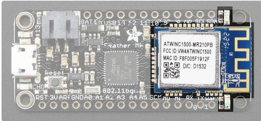
Since not all pins can be brought out to breakouts, due to the small size of the Feather, we use these to control the WiFi module
