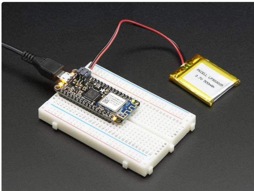
To make it easy to use for portable projects, we added a connector for any of our 3.7V Lithium polymer batteries and built in battery charging. You don't need to use a
