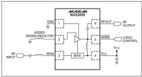
Figure 1. Typical application circuit for increased linearity.
