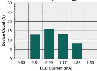
**Typical  $I_F$  for Switch Dropout**
