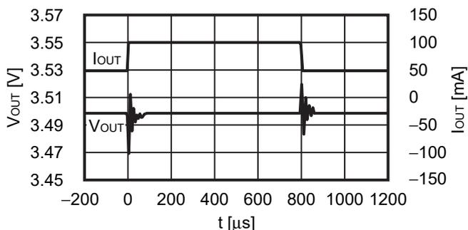
V<sub>IN</sub> = 4.5 V, C<sub>IN</sub> = C<sub>L</sub> = 2.2 μF, I<sub>OUT</sub> = 100 mA ↔ 500 mA
