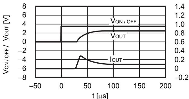
V<sub>IN</sub> = 3.5 V, C<sub>IN</sub> = C<sub>L</sub> = 2.2 μF, C<sub>SS</sub> = 0 nF, I<sub>OUT</sub> = 1000 mA,
