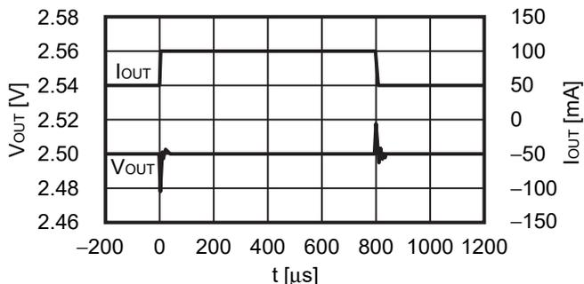
V<sub>IN</sub> = 3.5 V, C<sub>IN</sub> = C<sub>L</sub> = 2.2 μF, I<sub>OUT</sub> = 100 mA ↔ 500 mA
