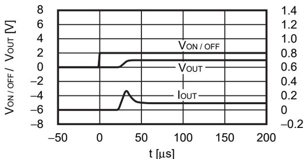
V<sub>IN</sub> = 2.0 V, C<sub>IN</sub> = C<sub>L</sub> = 2.2 μF, C<sub>SS</sub> = 0 nF, I<sub>OUT</sub> = 1000 mA,
