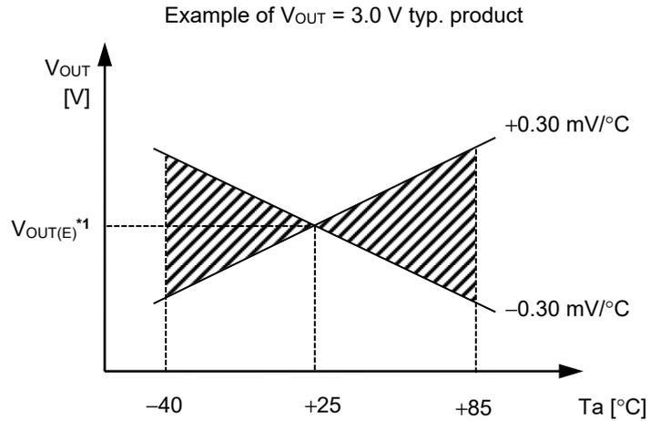
\*1.  $V_{OUT(E)}$  is the value of the output voltage measured at  $T_a = +25^{\circ}$ C.
