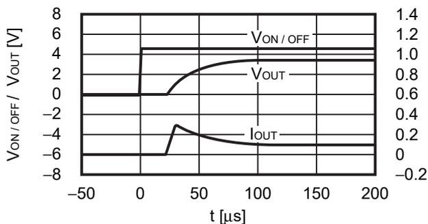
V<sub>IN</sub> = 4.5 V, C<sub>IN</sub> = C<sub>L</sub> = 2.2 μF, C<sub>SS</sub> = 0 nF, I<sub>OUT</sub> = 1000 mA,
