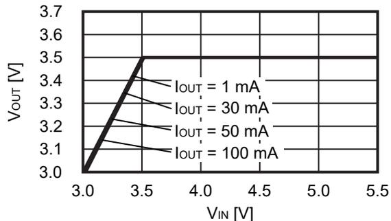
**3. Dropout voltage vs. Output current**
